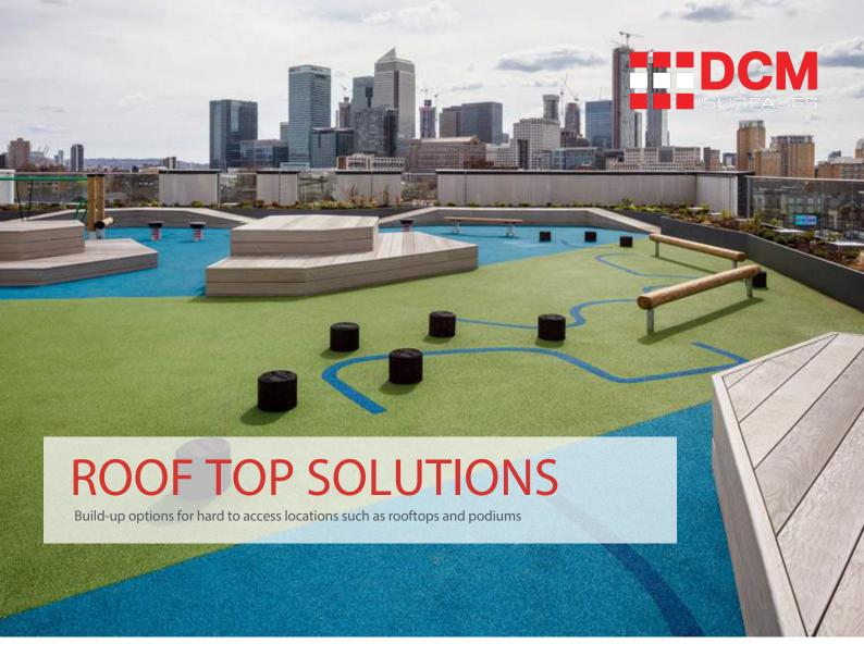
Unlike typical ground-level installations, which require tarmac or MOT stone sub-bases, roof-tops require a light-weight, cold-applied material which can easily be manouvered into position.
